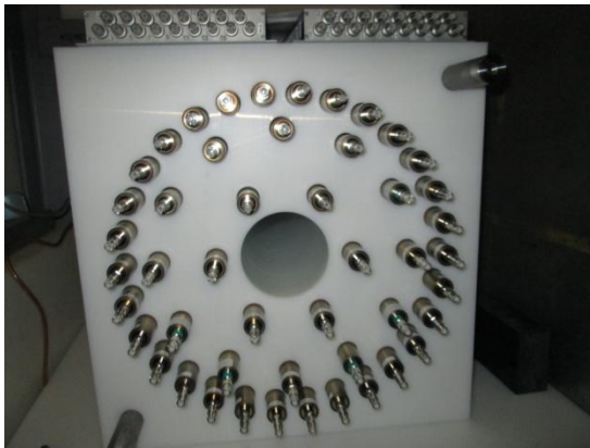
Counters embedded in a polyethylene matrix (version with 48 counters)
