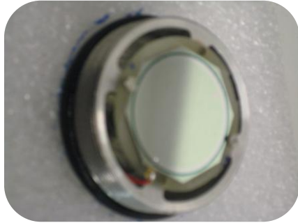
Silicon detector was located in front of the tape
